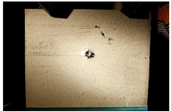
Fig.4. Tested sample after 1 shot penetration.
