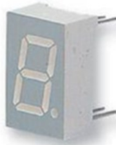
Figure 7-24. A Typical Seven-Segment Display
