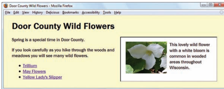
Figure 13.4 The white scrolling area on the page is an inline frame that displays a separate web page
