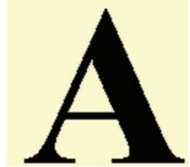
Figure 5.24 This graphic was not antialiased: The letter "A" has a jagged look
