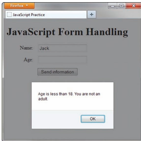
Figure 14.20 The validateform.html file displayed in the browser with input in the Name box and without input in the Age box; the alert message appears after the submit button is clicked
