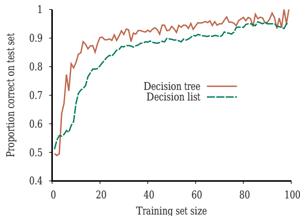
Figure 19.12 Learning curve for DECISION-LIST-LEARNING algorithm on the restaurant data. The curve for LEARN-DECISION-TREE is shown for comparison; decision trees do slightly better on this particular problem.
