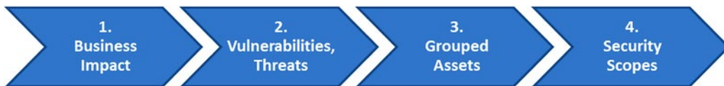
Figure 4-6. Security scopes can be identified using a four-step process, starting with the business impact of a failure and working backward through the risk to group assets into a common security scope.
