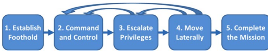
Figure 1-6. The Enterprise Cybersecurity Attack Sequence consists of a series of five steps involved in cyberintrusions. Steps 2 through 4 may cycle multiple times as attackers move around and obtain privileges in the target environment.
