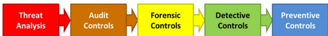
Figure 11-5. The Audit First Methodology involves starting from the threat analysis and then designing controls to counter those threats, beginning with audit controls, then forensic controls, detective controls, and finally preventive controls.
