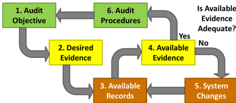
Figure 11-2. Starting with the cybersecurity audit objective, this audit process is followed to identify the evidence necessary to satisfy the audit objective. The audit process may involve modifying IT systems or manual processes to log additional data.
