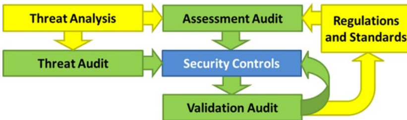
Figure 11-3. Among many audit types, there are three main cybersecurity audit types: threat, assessment, and validation.
