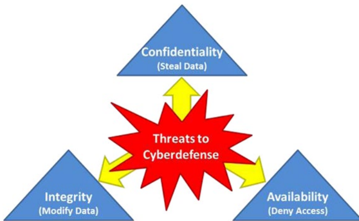
Figure 1-2. The damage caused by threats to cyberdefense can be characterized by losses of confidentiality, integrity, or availability.
