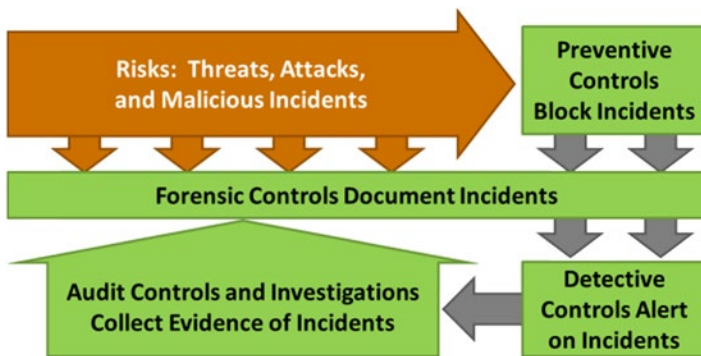
Figure 2-7. Interactions among risks and the different types of controls. While preventive controls are the controls that actually stop the risks, the other controls are critical to making people aware an incident is occurring so they can investigate, contain, and remediate the incident.
