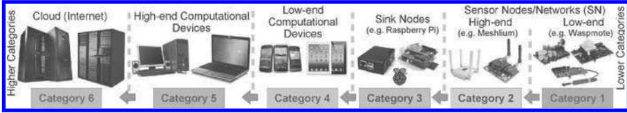
Figure 3.17: Categorization of CPS devices based on their computational capabilities. The devices belonging to each category have different capabilities depending on processing, memory, and communication. From left to right, the devices become more and more expensive; the computational capabilities also increase.
