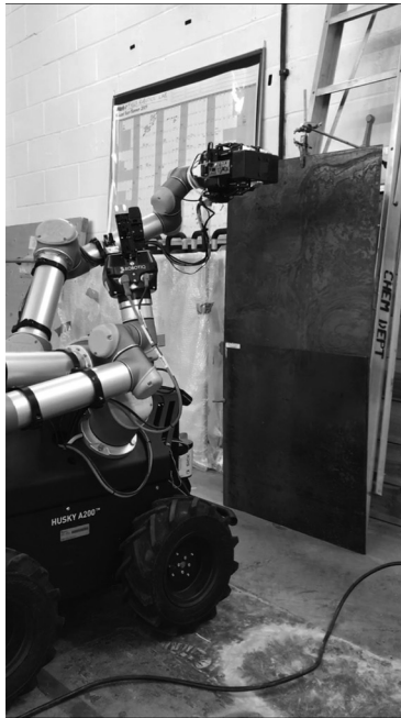
Figure 13.24: Dual UR5 husky A200 with the FMCW millimetre-wave sensor in the gripper during a corrosion inspection.
