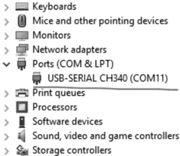
Figure 6.7: Serial communication port associated with the interface module.
