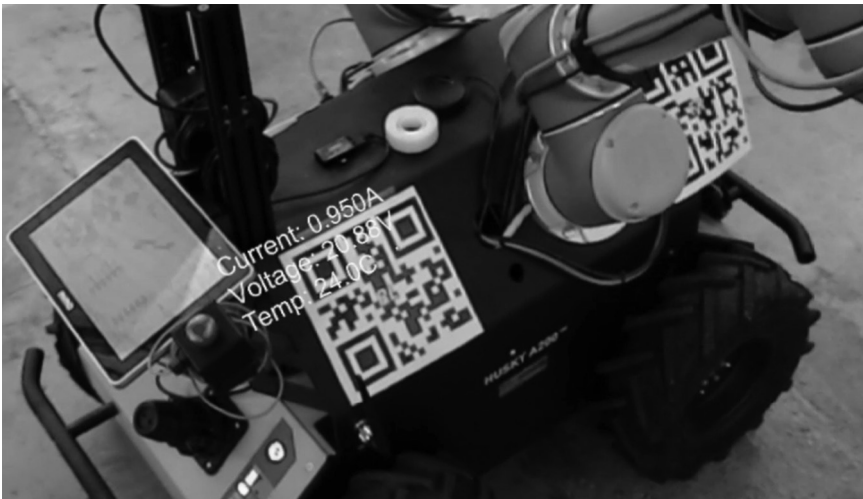
Figure 13.22: QR codes are recognized by an MR device and enable human-readable health status information to be overlaid on the robotic platform.
