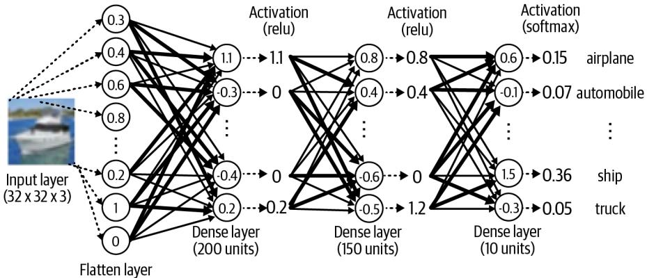
Figure 2-5. A diagram of the MLP architecture
