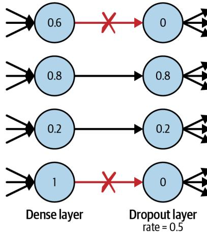
Figure 2-15. A dropout layer
