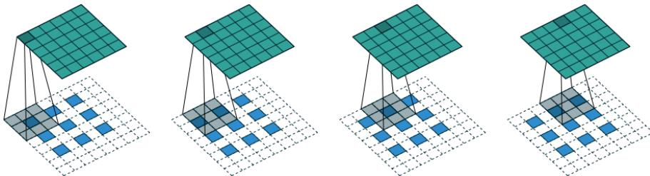
*Figure 3-5. A convolutional transpose layer example (source: Dumoulin and Visin, 2018)<sup>2</sup>*
