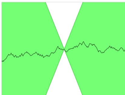
Figure 4-11. A Lipschitz continuous function (source: [Wikipedia](#))
