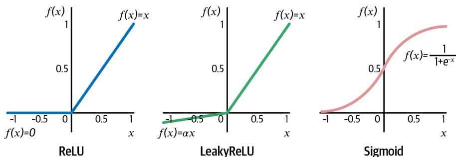
Figure 2-6. The ReLU, LeakyReLU, and sigmoid activation functions
