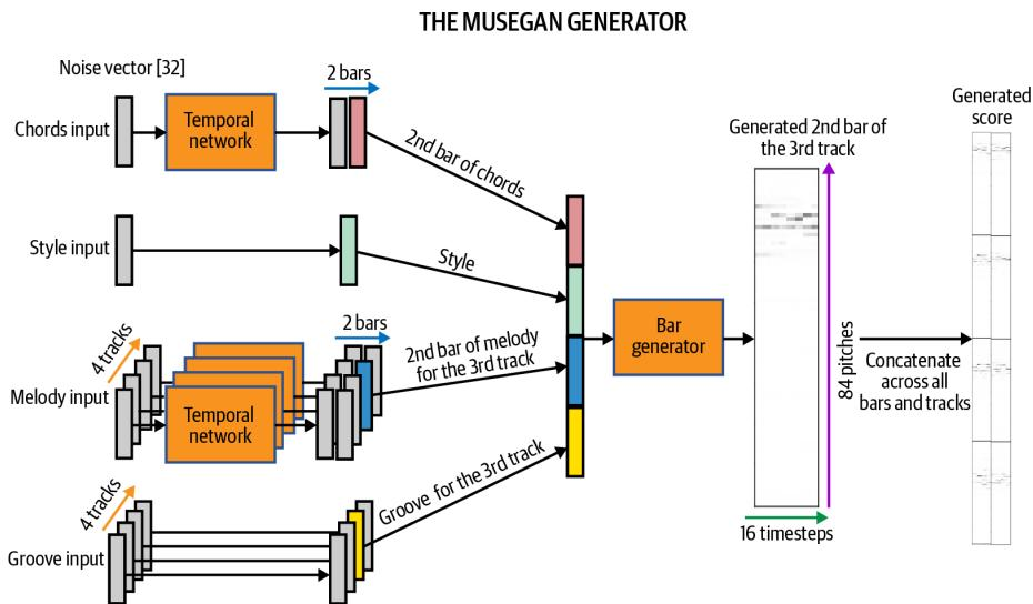
Figure 11-15. High-level diagram of the MuseGAN generator
