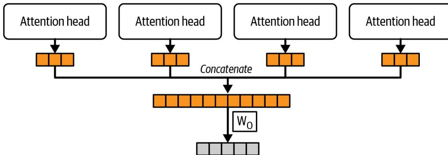
Figure 9-3. A multihead attention layer with four heads
