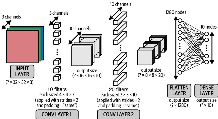
*Figure 2-13. A diagram of a convolutional neural network*
