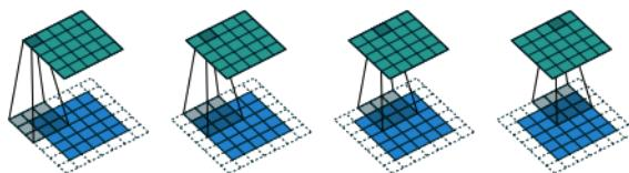
Figure 2-12. A  $3 \times 3 \times 1$  kernel (gray) being passed over a  $5 \times 5 \times 1$  input image (blue), with `padding = "same"` and `strides = 1`, to generate the  $5 \times 5 \times 1$  output (green) (source: Dumoulin and Visin, 2018)<sup>5</sup>
