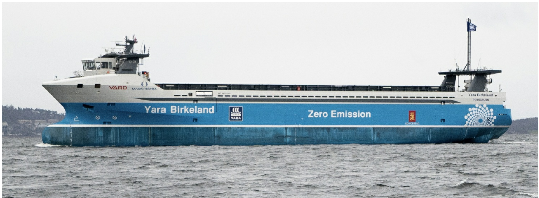
Figure 7.4. Autonomous, electric containership YARA BIRKELAND.
