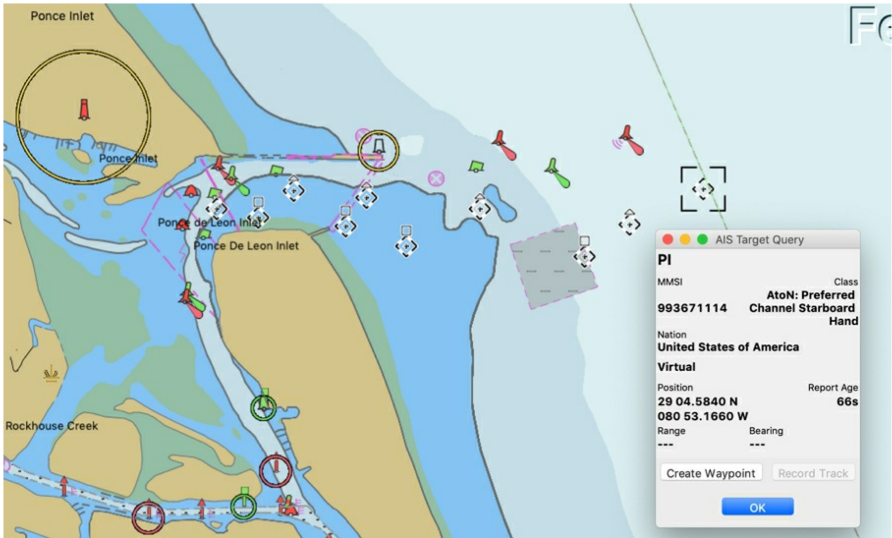
Figure 6.3. AIS display of real ATONs and fake virtual ATONs in Ponce De Leon Inlet, Florida.
