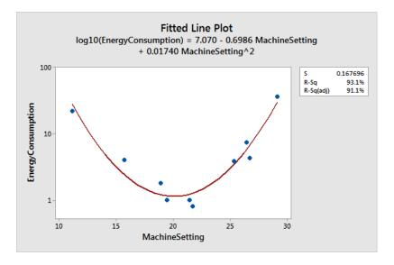
The chart displays the relationship between machine setting and energy consumption. Notice how the effect of machine setting on mean energy usage depends on where you are on the fitted curve. On the xaxis, if you begin with a setting of 12 and increase it by 1, energy consumption decreases. On the other hand, if you start at 25 and increase the setting by 1, energy consumption increases. Near 20 and consumption doesn't change much.
