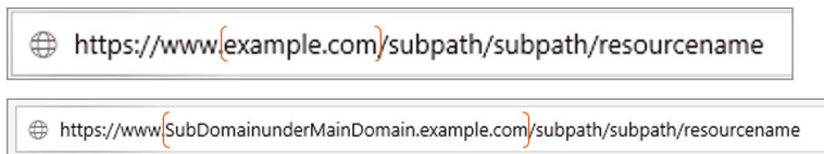
FIGURE 13-2 Two examples of URLs with the DNS domain portion highlighted between the brackets.
