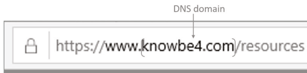
FIGURE 13-7 An example of a URL with the DNS domain highlighting between brackets.
