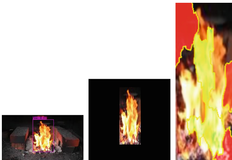
Fig. 8. LIME visual explanation for fire with 8 features: model predictions (left); cropped input image (middle); Zoomed explanation (right)
