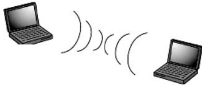
Figure 18: Peer-to-peer wireless network.
