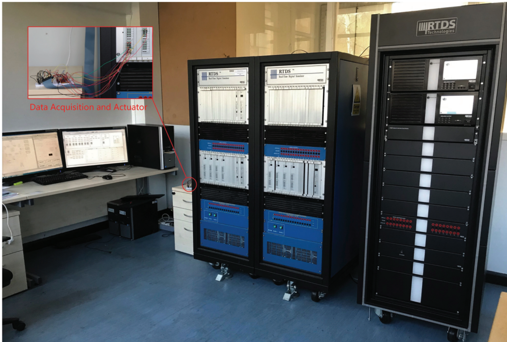
Figure 5.15 Interactions between MATLAB ® , Real-Time Digital Simulator, and Data Acquisition and Actuator module. After performing the conditional random field-based reinforcement learning using MATLAB, the scheduling results are transmitted back to Real-Time Digital Simulator using the Giga-Transceiver Analogue Input Card. Meanwhile, real-time operating signals are transmitted from Real-Time Digital Simulator to MATLAB using the Giga-Transceiver Analogue Output Card.
