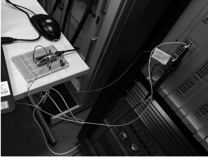
Figure 8.10 An example of hardware-based interfacing technique with the microcontroller MBED .
