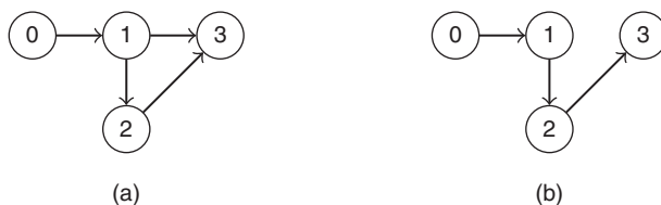
Figure 6.3 The attack graphs under different network topologies. (a) Attack graph under topology A. (b) Attack graph under topology B.
